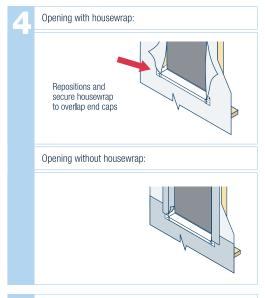
Install waterproofing in shingle fashion, including over jamb and head flashing. PROVIDE FREE DRAINAGE FOR SURESILL $^{TM}$ .
