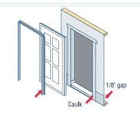
IMPORTANT: Allow 1/8" gap behind window or door threshold
